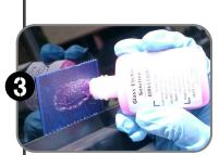
Carefully dab etching solution over the numbers on each stencil tissue. Avoid putting the solution too close to the edge of the stencil tissue since any accidental contact with the glass surface will result in an etch.
